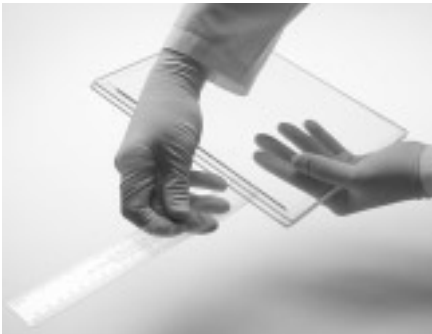
Fig 9A and B. IPG strip are loaded onto cassette and slid into place.
